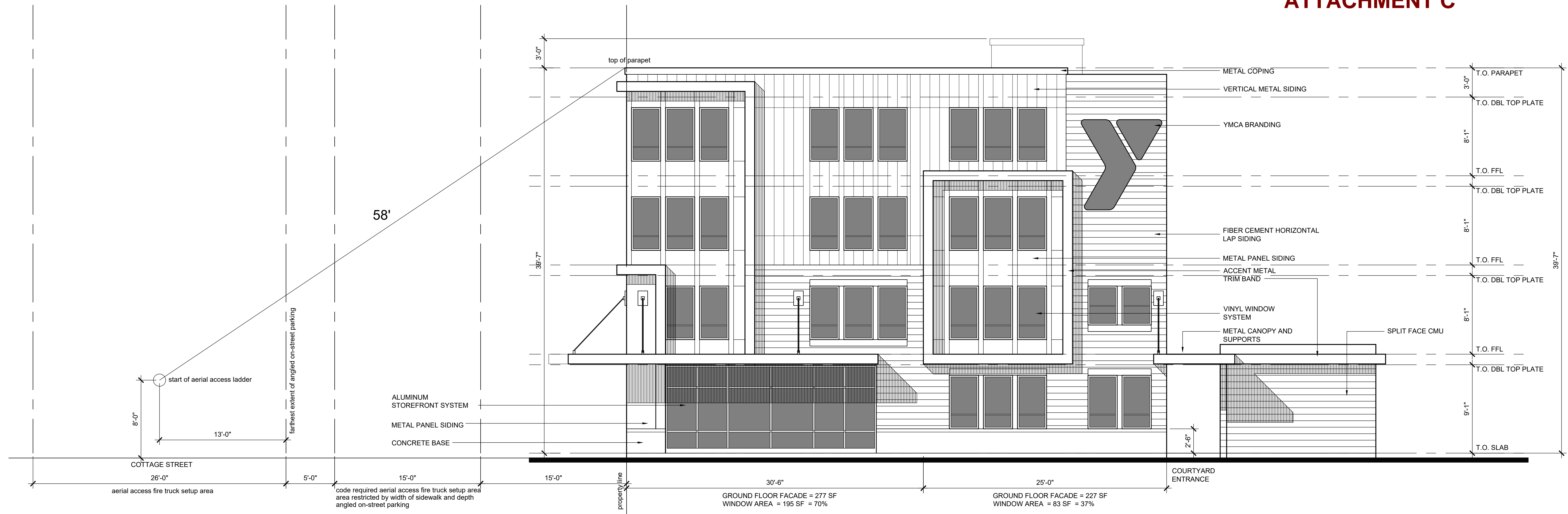
2 BUILDING ELEVATIONS - COURT ST NE A200 3/16" = 1'-0"
