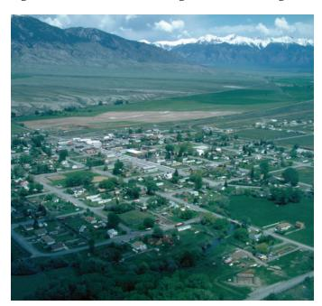
■ Figure 17. Aerial view of heavily damaged Mackay, Idaho. The unreinforced masonry buildings on the main commercial street of the small town were badly damaged in the 1983 Borah Peak, Idaho earthquake.
