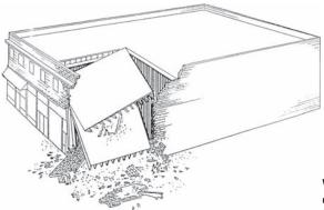
■ Figure 28. Failure of roof-towall connection, with resulting collapse. — Rutherford and Chekene
