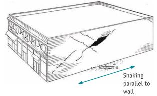
■ Figure 25. In-plane failure of unreinforced masonry walls. — Rutherford and Chekene
