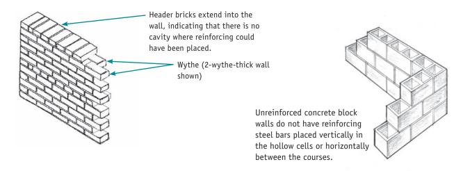
■ Figure 7. Components of unreinforced brick (left) and unreinforced concrete block (right) walls.
