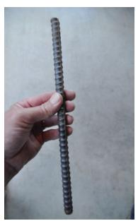
■ Figure 26. A piece of #4 bar (a steel reinforcing bar that is 4/8 inch in diameter).
