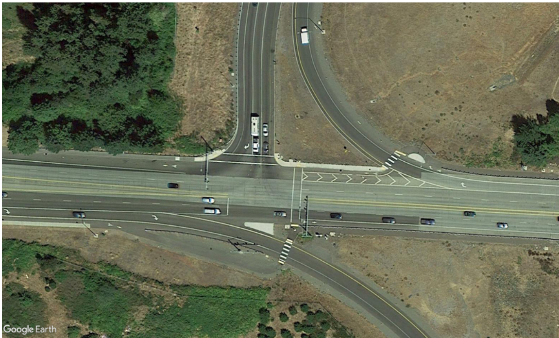
Aerial view of I-5 SB/Kuebler Boulevard intersection. The dual southbound right turn lanes are not behind an island as analyzed in the TIA.
