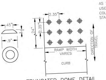
2'x4' MIN. DETECTABLE WARNING SURFACE. LOCATE IN THE LOWER 24" OF RAMP THROAT. ARRANGE DOMES USING IN-LINE PATTERN ONLY, AS SHOWN IN TRUNCATED DOME DETAIL. USE 2' x 2' TACTILE PANELS CENTERED IN RAMP. COLOR OF DETECTABLE SURFACE AREA TO BE RED. STANDARD BROOM FINISH ALL OTHER SIDEWALK AREAS.
