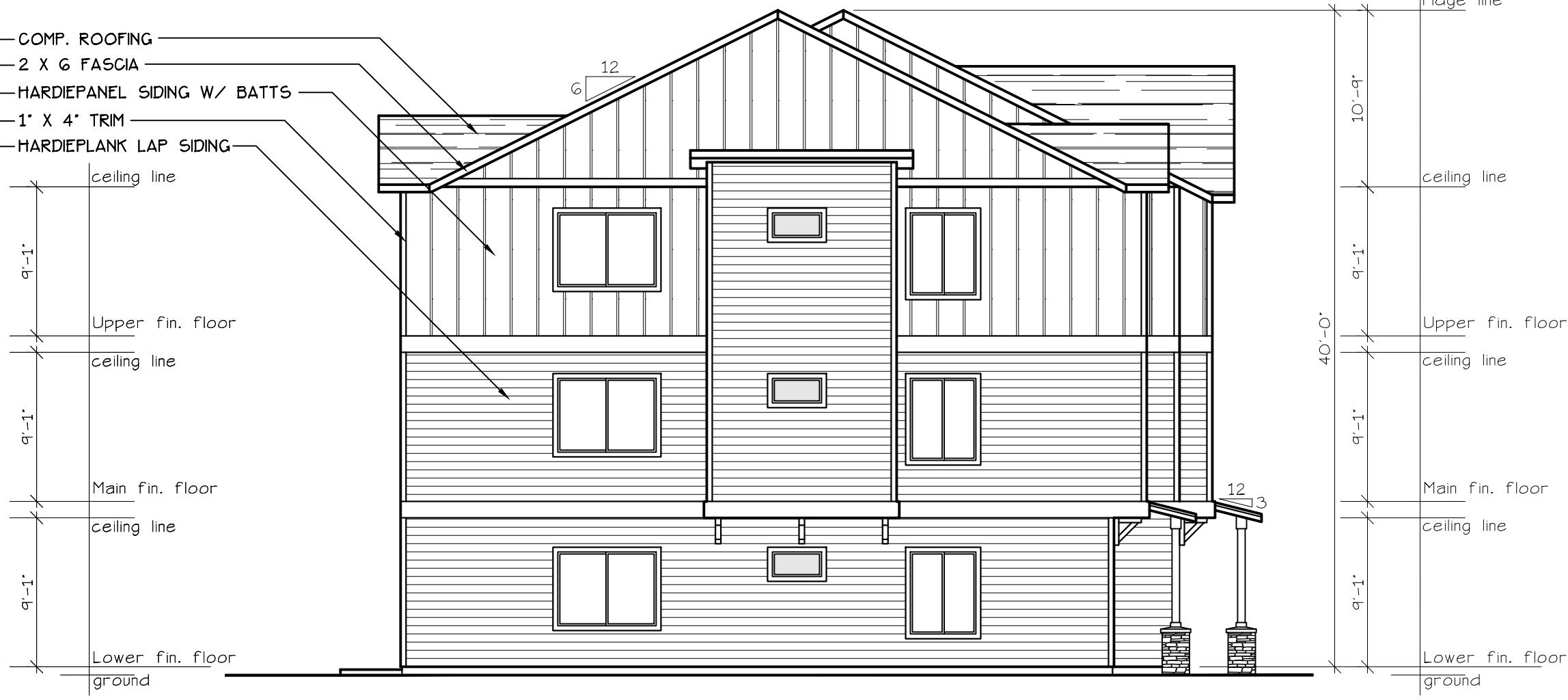
END ELEVATION (TYPE A UNITS) SCALE: 1/8" = 1'-0" (BLD. 18)
