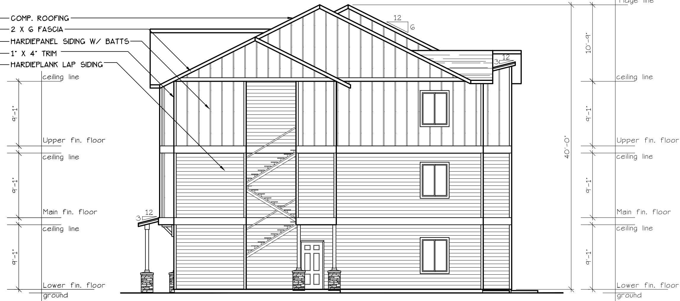
END ELEVATION (TYPE A UNITS) SCALE: 1/8" = 1'-0" (BLD. 18)
