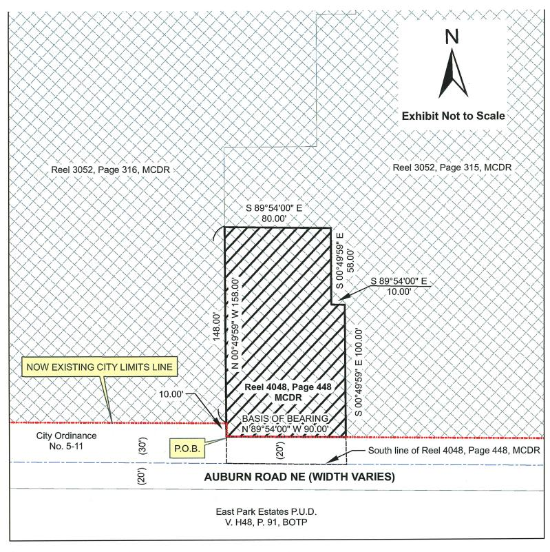
BASIS OF BEARING - North right-of-way of Auburn Road NE as shown on MCSR 37531.
