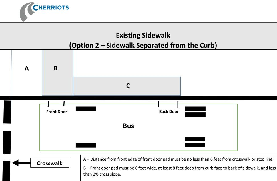
C – Rear door pad must extend at least 21 feet, 6 inches back from the front door pad and be 5 feet deep.
