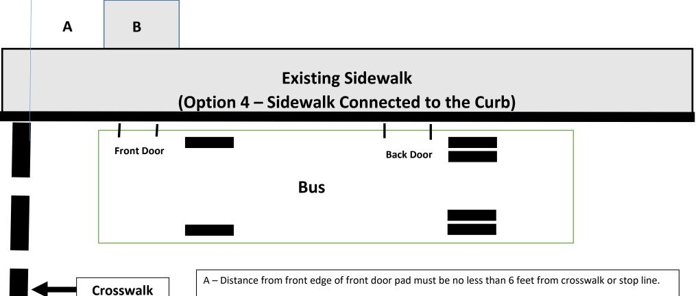
B – Front door pad must be 6 feet wide, and create at least 8 feet of depth from curb face to back the pad, and less than 2% cross slope.
