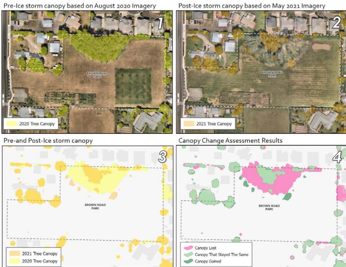
Figure 2. Tree canopy polygons (panels 1 & 2) were derived from high resolution imagery and 3D models using artificial intelligence technology, which then were intersected, analyzed, and compared (panel 3) to identify where canopy was lost, gained, and remained the same (panel 4).
