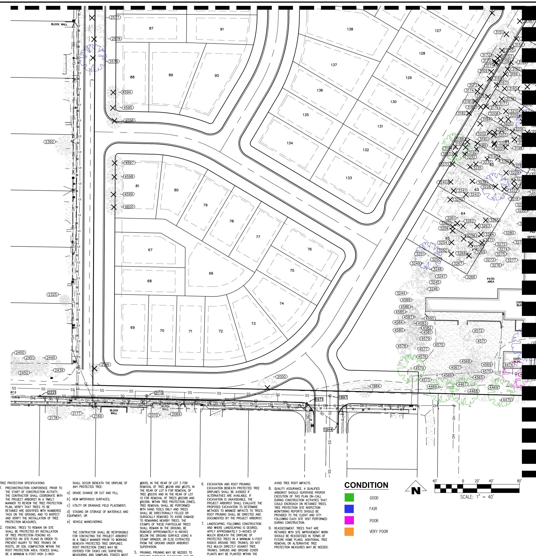
CHAIN LINK MESH SECURED TO METAL POSTS DRIVEN INTO THE GROUND. THE CONTRACTOR IS RESPONSIBLE FOR COORDINATING WITH THE PROJECT ARBORIST PRIOR TO OPENING, ADJUSTING OR REMOVING TREE PROTECTION FENCING. TREE PROTECTION ZONE. WITHOUT AUTHORIZATION FROM THE PROJECT ARBORIST, NONE OF THE FOLLOWING
