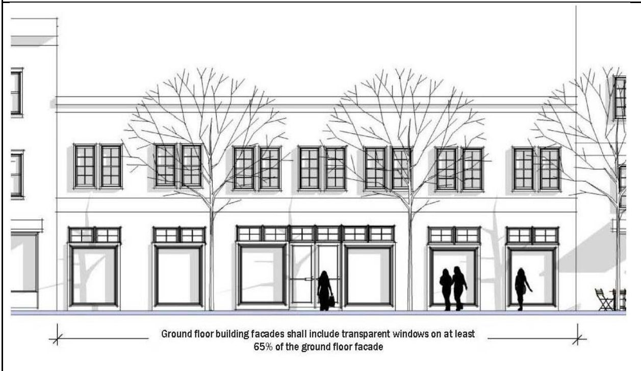
FIGURE 533-5 GROUND FLOOR WINDOWS
