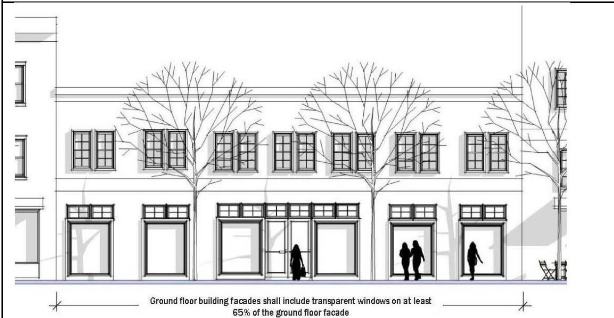
FIGURE 536-5 GROUND FLOOR WINDOWS
