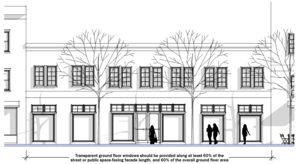
FIGURE 524-4. GROUND FLOOR WINDOWS
