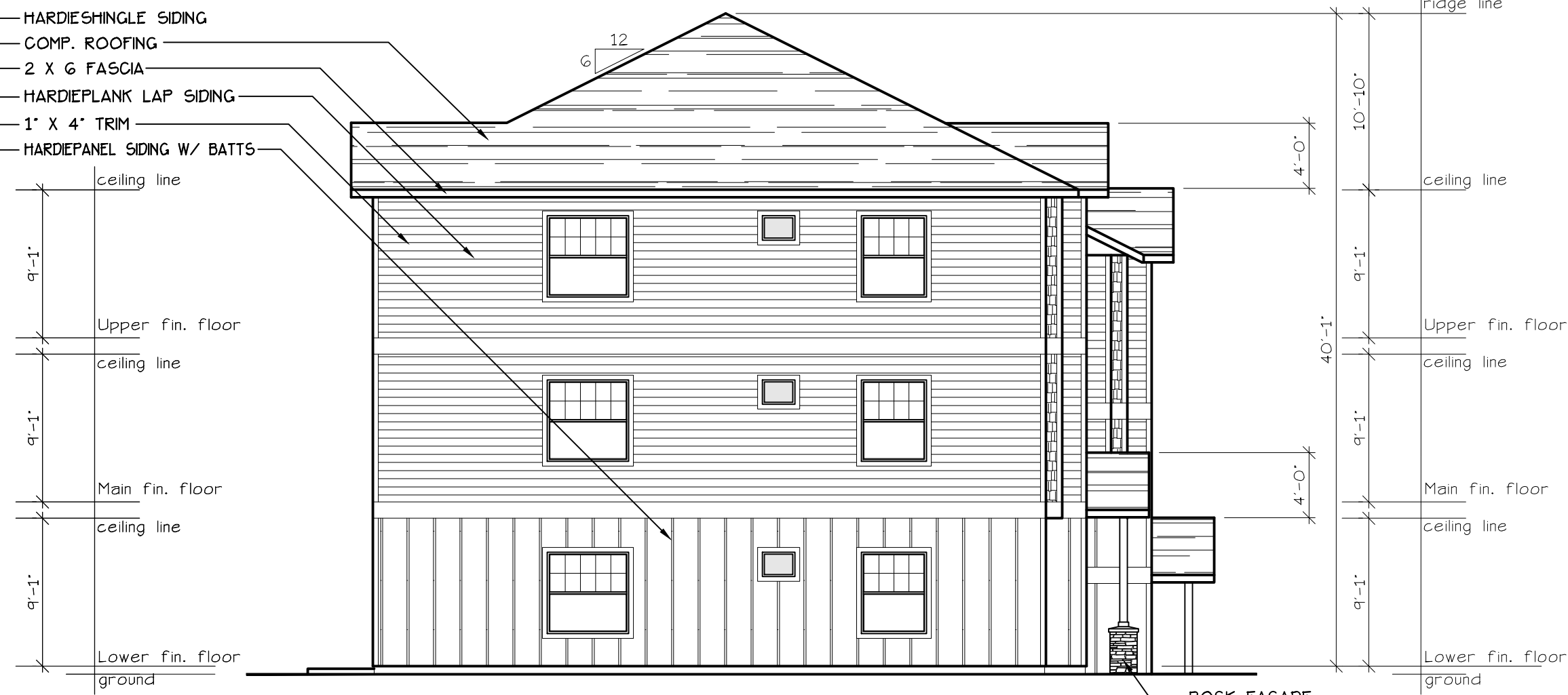
SOUTH ELEVATION (TYPE C UNITS) SCALE: 1/8" = 1'-0" BLD. 12
