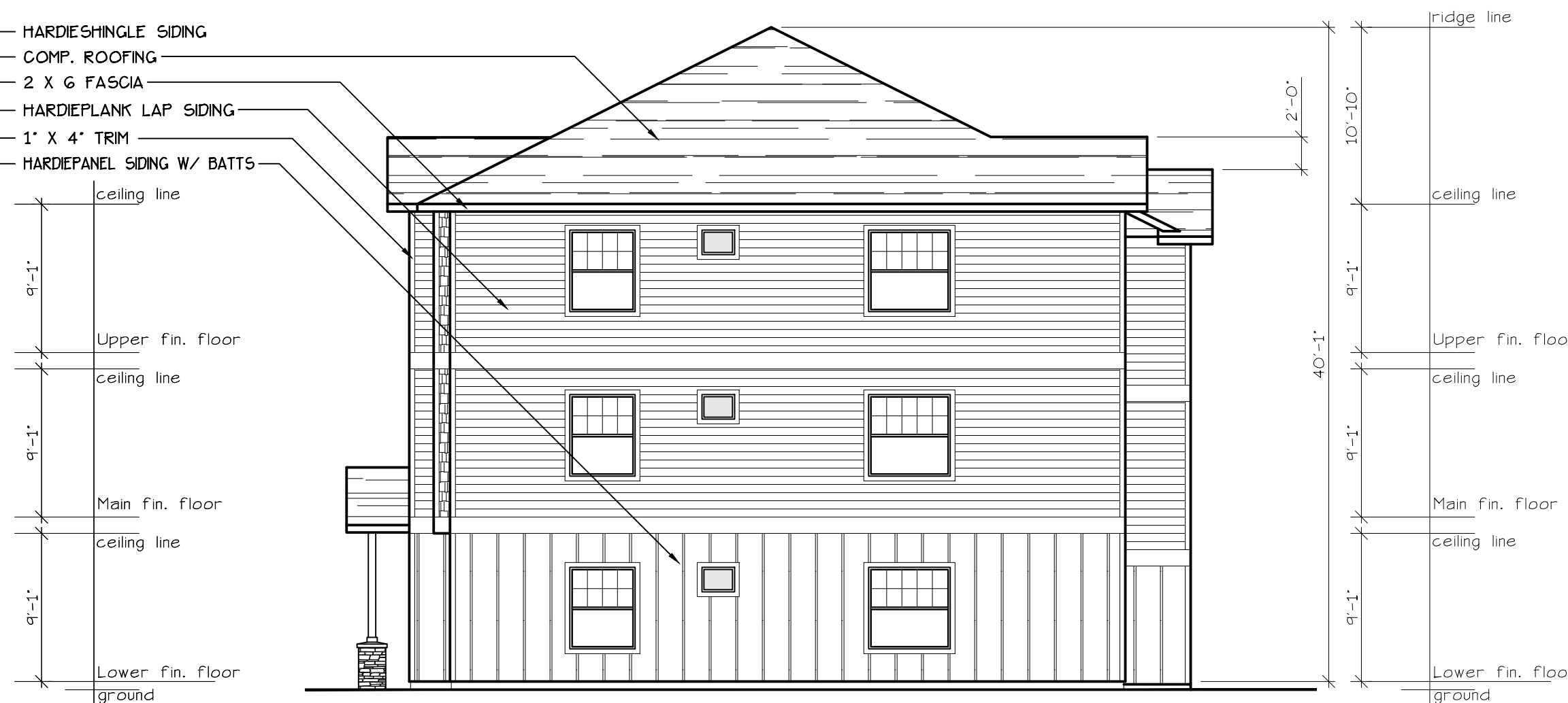
WEST ELEVATION (TYPE C UNITS) SCALE: 1/8" = 1'-0" BLD. 1
