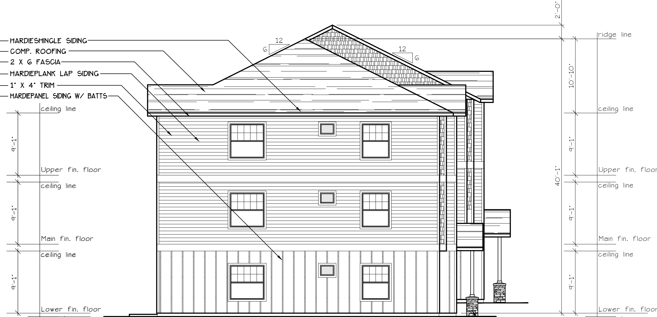
EAST ELEVATION (TYPE C UNITS) SCALE: 1/8" = 1'-0" BLD. 1
