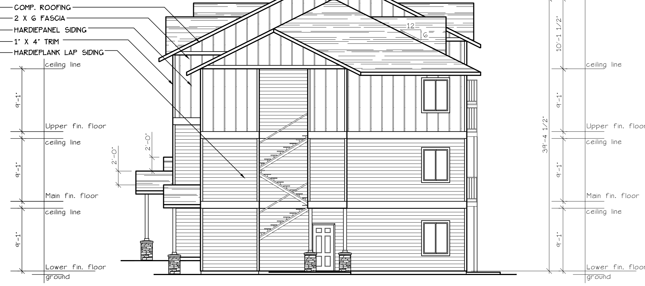
WEST ELEVATION (TYPE A1 UNITS) SCALE: 1/8" = 1'-0" BLD. 13
