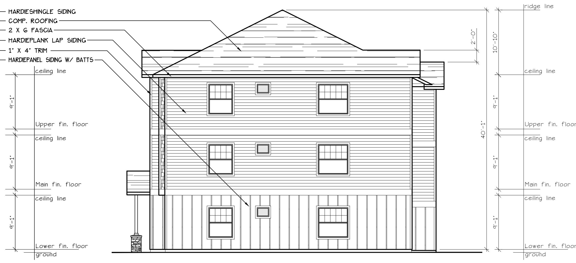
WEST ELEVATION (TYPE C UNITS) SCALE: 1/8" = 1'-0" BLD. 1
