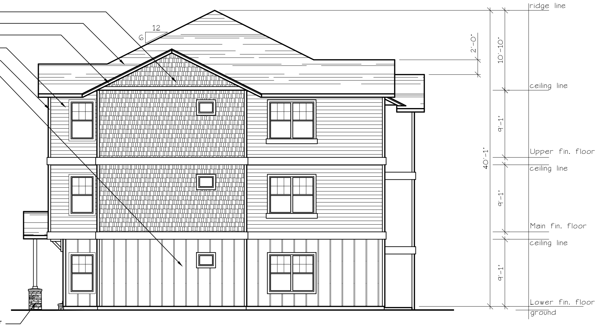
WEST ELEVATION (TYPE A2 UNITS) SCALE: 1/8" = 1'-0" (BLD. 3)
