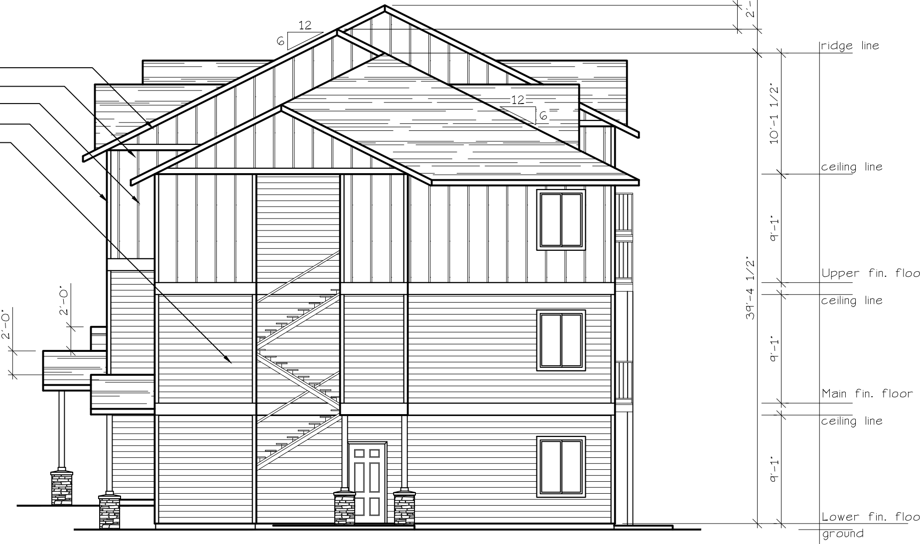
WEST ELEVATION (TYPE A1 UNITS) SCALE: 1/8" = 1'-0" BLD. 13
