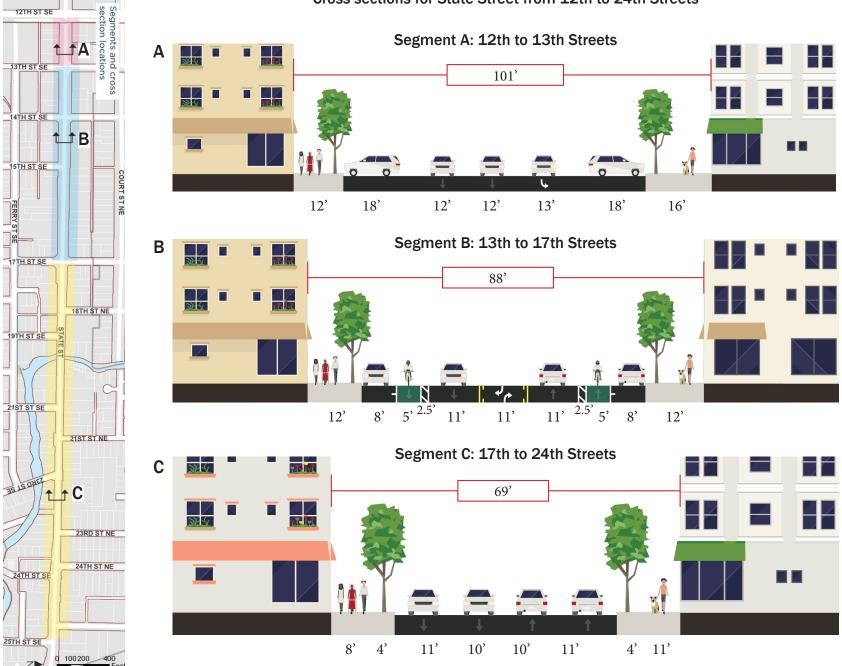
Note: The proposed design of State Street between 13th to 14th street does not include bike lanes. It has one lane in each direction and a center turn lane, and it provides wider sidewalks and on-street parking.
