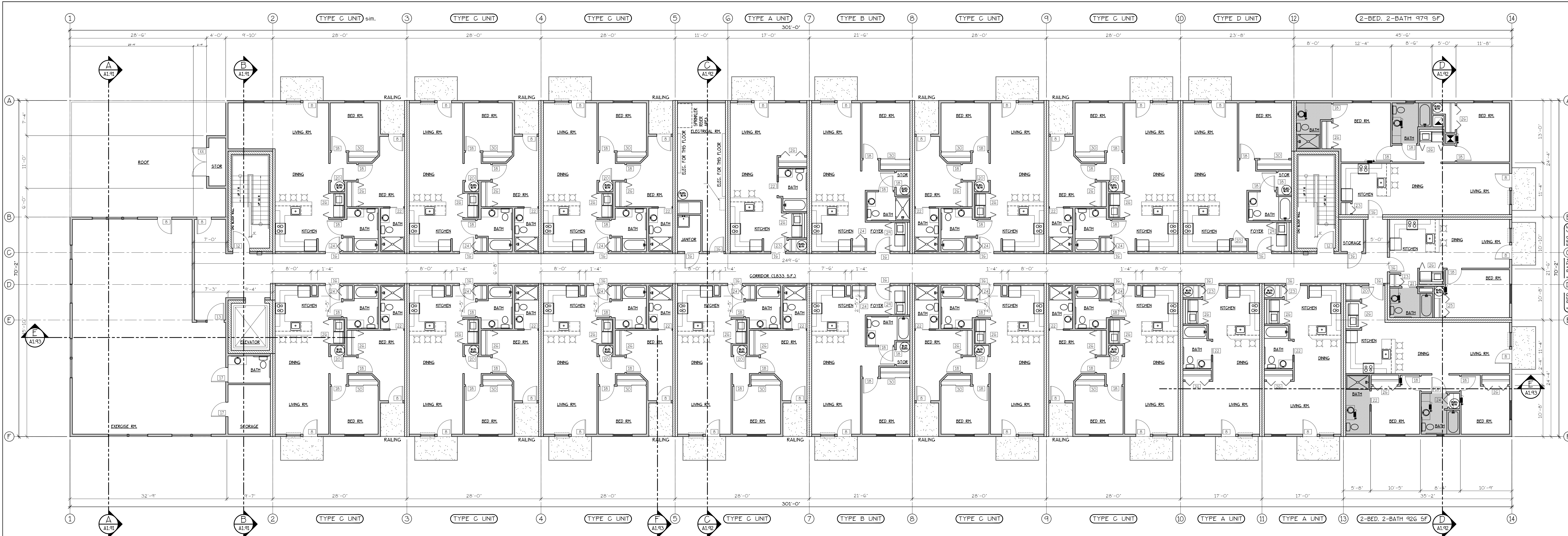
FOURTH FLOOR PLAN SCALE: 1/8" = 1'-0" CHANDICAP ADAPTABLE/ACCESSIBLE FOURTH FLOOR AREA = 20,373 S.F. FOURTH FLOOR COMMON SPACE = 2,096 S.F.
