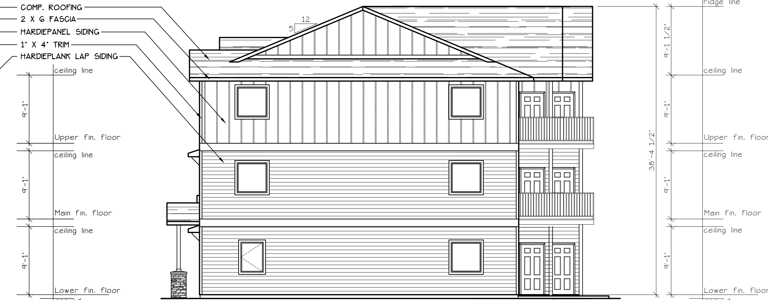
EAST ELEVATION (TYPE C UNITS) SCALE: 1/8" = 1'-0" (BLD. 9.14.20.+33)
