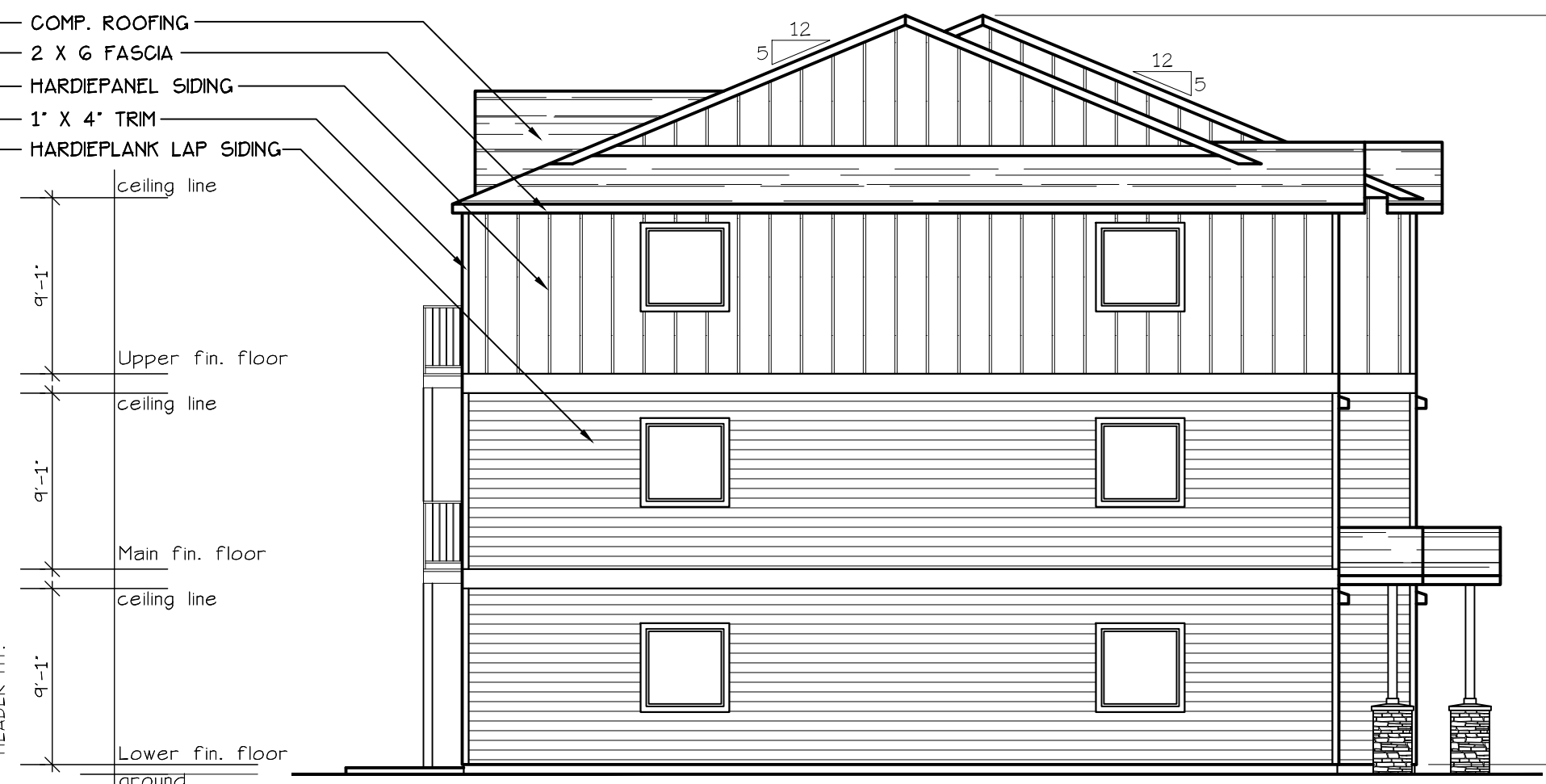
NORTH ELEVATION (TYPE B UNITS) SCALE: 1/8" = 1'-0" BLD. 13,19,23,26,+29
