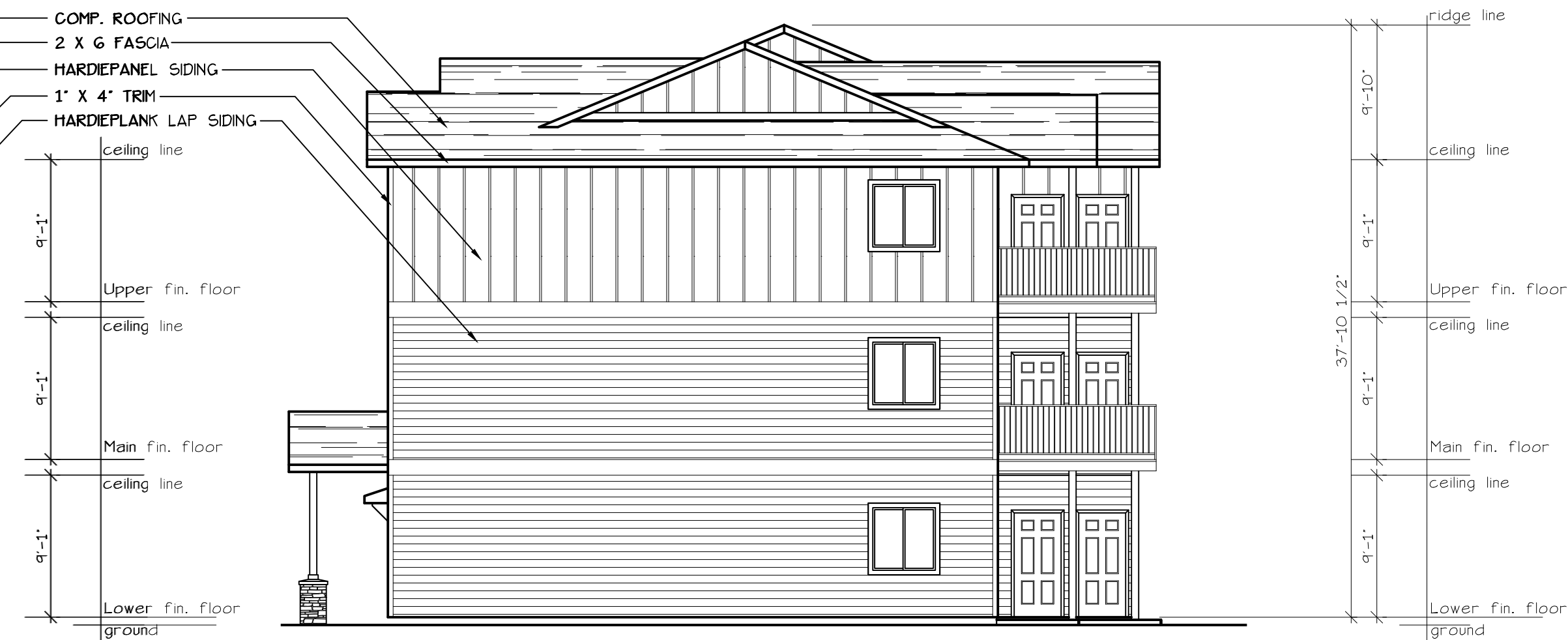
NORTH ELEVATION (TYPE D UNITS) SCALE: 1/8" = 1'-0" (BLD. 15 + 36)
