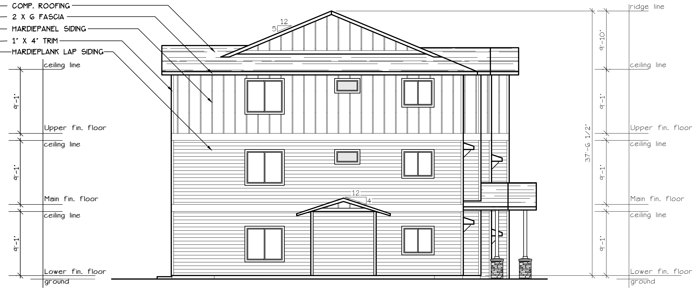
SOUTH ELEVATION (TYPE E UNITS) SCALE: 1/8" = 1'-0" BLD. 27
