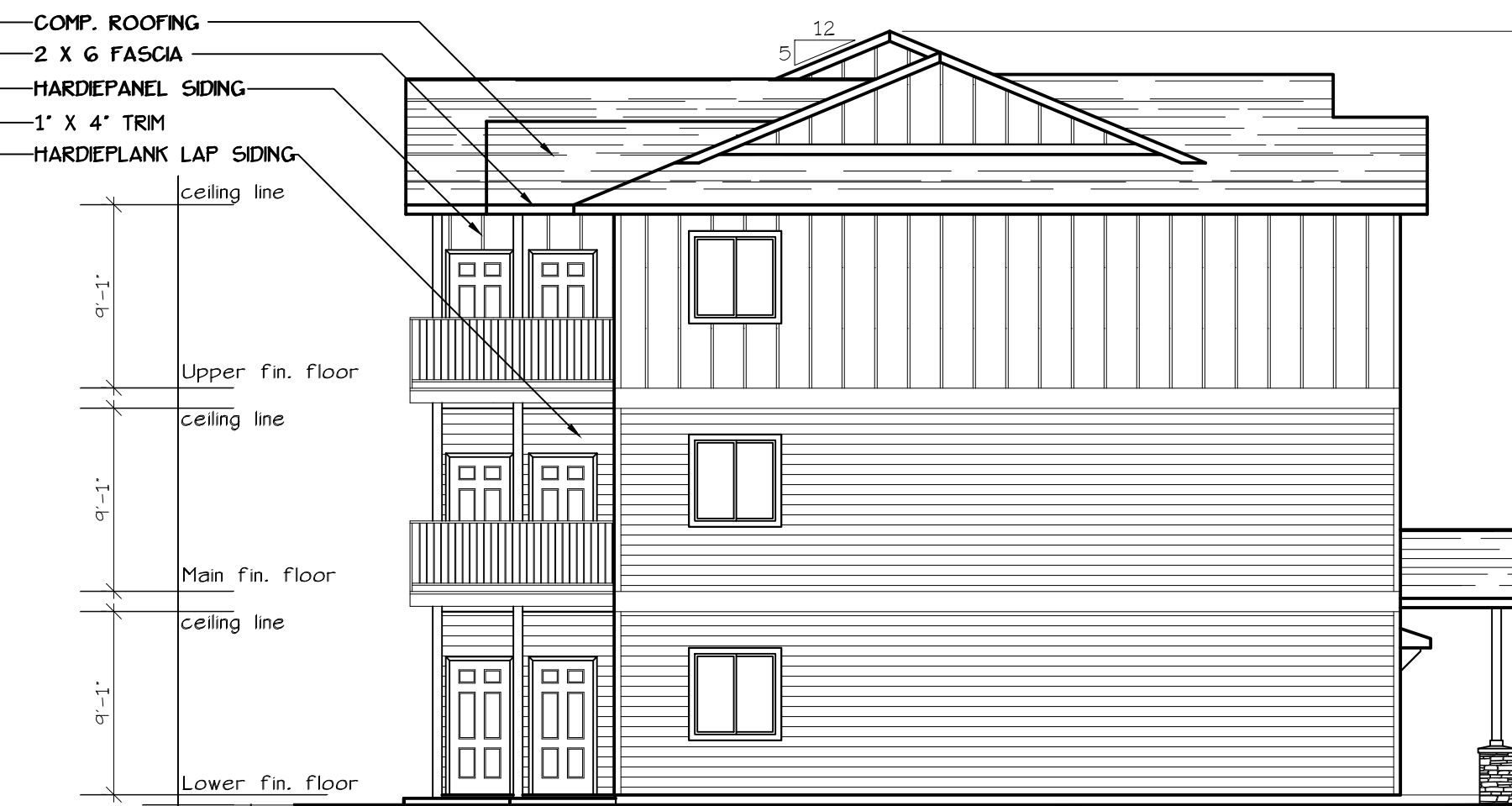
SOUTH ELEVATION (TYPE D UNITS) SCALE: 1/8" = 1'-0" (BLD. 1.4.16.17.18.+35)
