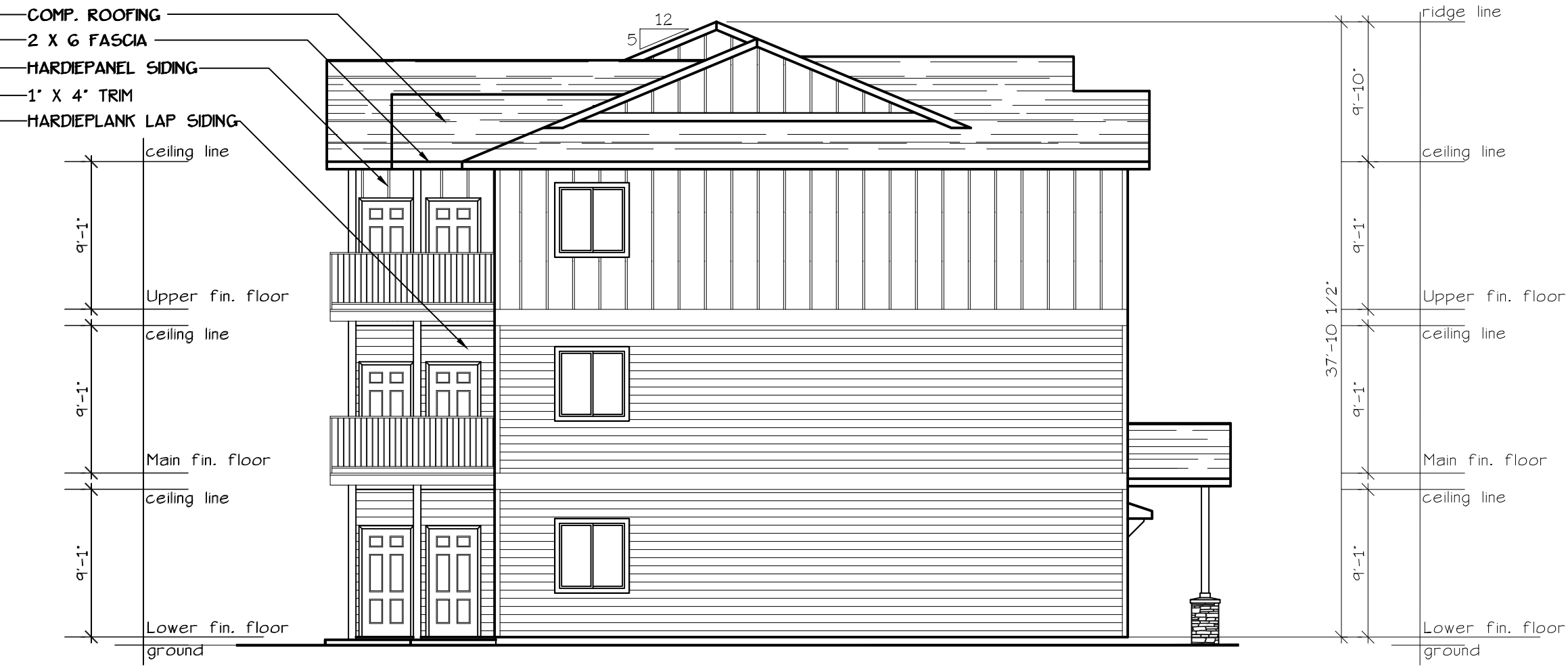
SOUTH ELEVATION (TYPE D UNITS) SCALE: 1/8" = 1'-0" (BLD. 15 + 36)
