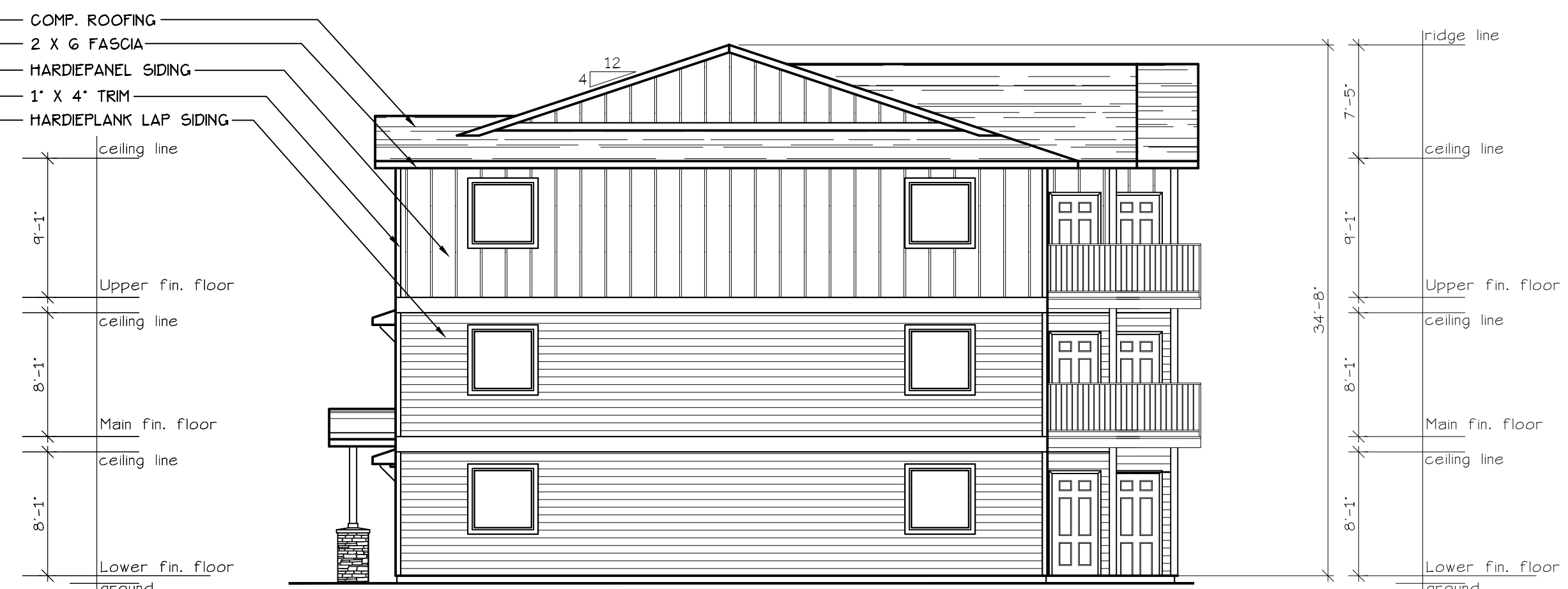
NORTH ELEVATION (TYPE C UNITS) SCALE: 1/8" = 1'-0" BLD. 2.11.22.32.+34
