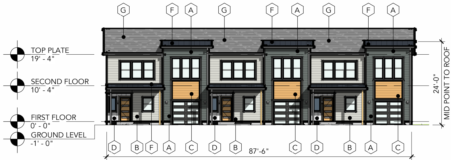
1 BUILDING TYPE 1 - FRONT ELEVATION
