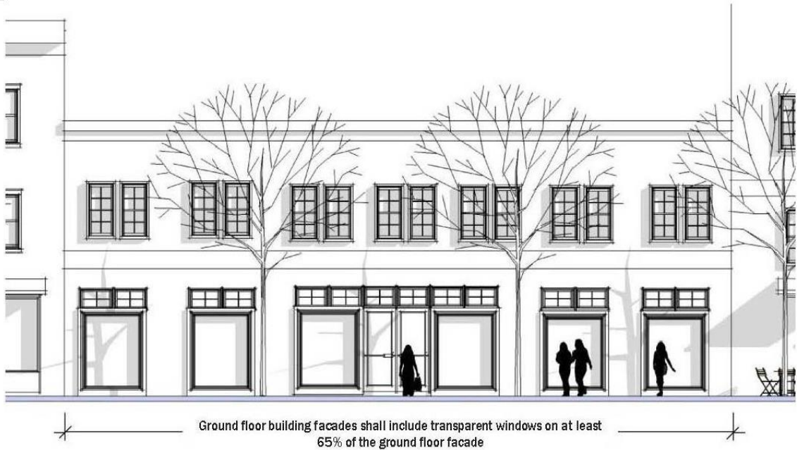
FIGURE 536-5 GROUND FLOOR WINDOWS
