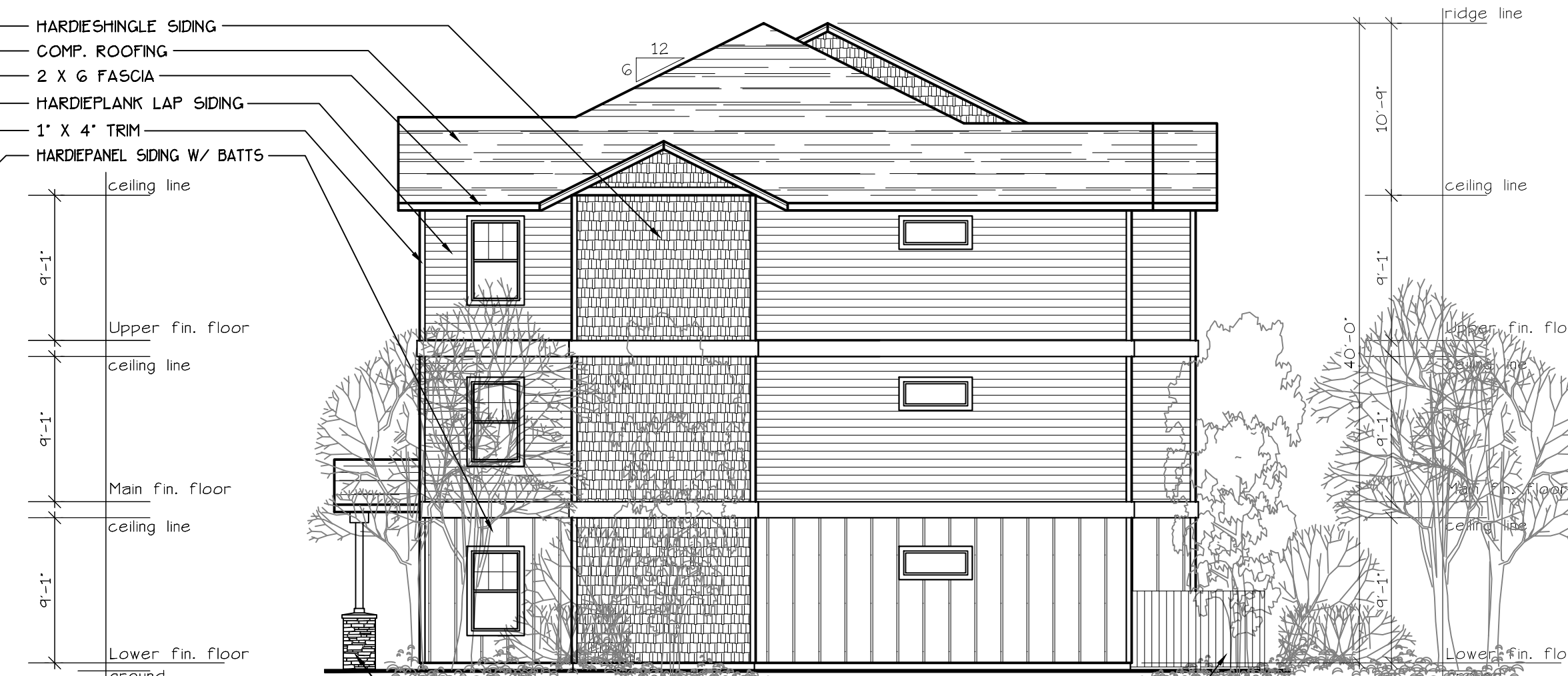
ROCK FACADE | TYPE B UNITS | 5' HIGH PRIVACY FENCE WEST ELEVATION (BLD. 10) SCALE: 1/8" = 1'-0"
