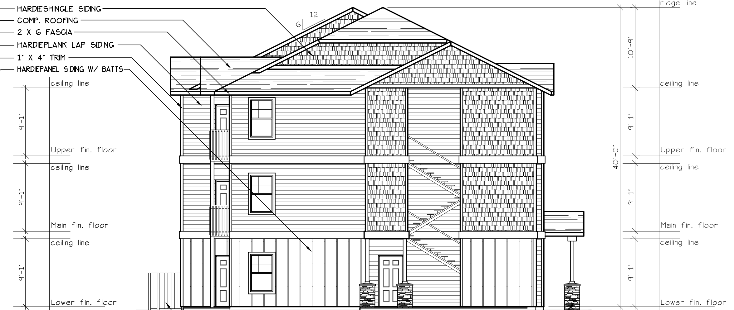
5' HIGH PRIVACY FENCE | TYPE A UNITS | ROCK FACADE EAST ELEVATION (BLD. 10) SCALE: 1/8" = 1'-0"
