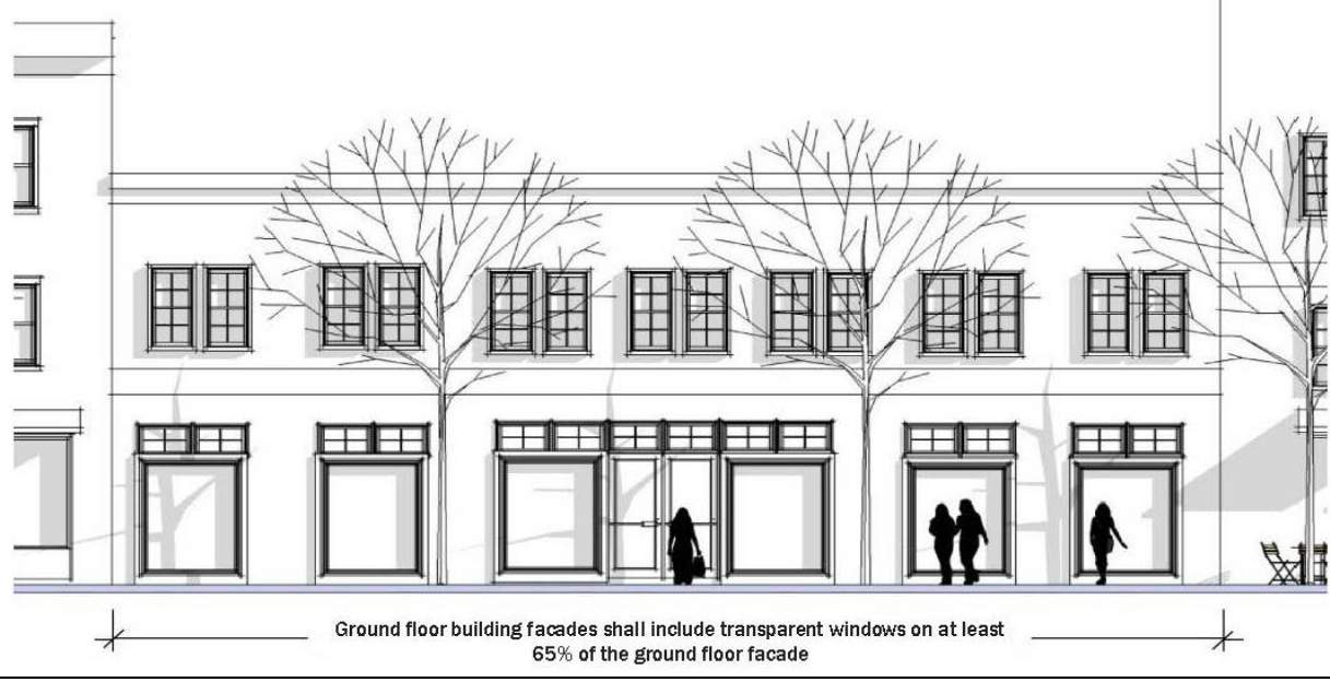
FIGURE 533-5 GROUND FLOOR WINDOWS
