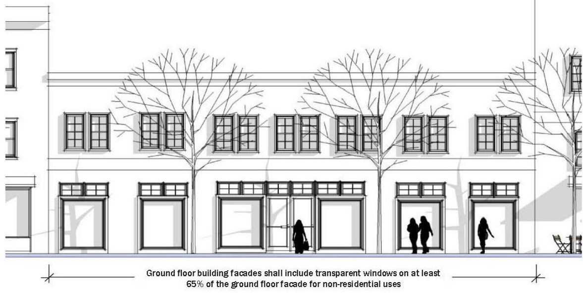
FIGURE 534-5 GROUND FLOOR WINDOWS
